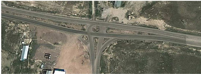
At-grade Intersection between Two Class II Roads (AH1 and AH84) in Turkey (Google Earth 201106)
